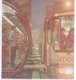
Top left, centre left and above right: biarticulated Volvo buses stop to pick up passengers waiting in bus tubes, which speed the boarding process. People using wheelchairs can enter the tubes via a lift. Photos: © Volvo Bus Image Gallery – Website: www.volvo.com Centre: Mayor Jaime Lerner. Photo: © Jaime Lerner – Website: www.jaimelerner.com
